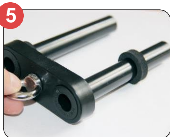
5 Place neoprene washers on to tubes, connect eyebolt and insert fitting into holes.
