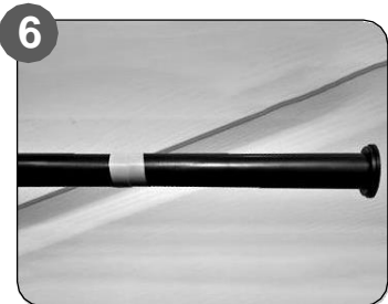
6 If longer depth is required multiple EX tubes can be used, and secured together with insulation tape to improve insertion.
